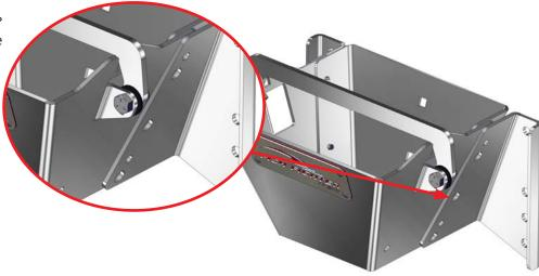
**3.** Install using (2)  $\frac{1}{4}$ " Cap Screw and (2) Nylock Nuts per side.
